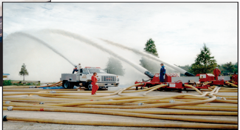
October 29, 1997 — a coordinated effort of Hired Gun Gang members records industry's largest documented firewater flow of 29,567 gpm using large volume pumps, guns, and hose.
