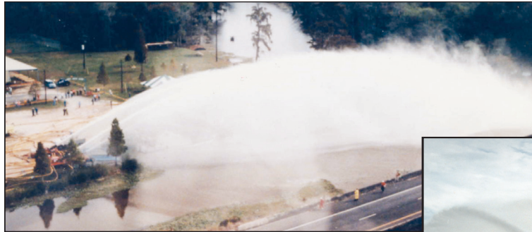
October 29, 1997 — a coordinated effort of Hired Gun Gang members records industry's largest documented firewater flow of 29,567 gpm using large volume pumps, guns, and hose.
