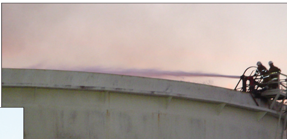
A rim-mount Dasplit™ Tool is deployed for safe and effective reach to quickly extinguish seal fire
