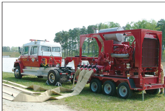
DPAT 6040 - 6,000 gpm transportable pump with a pumping capacity of 150 psi
