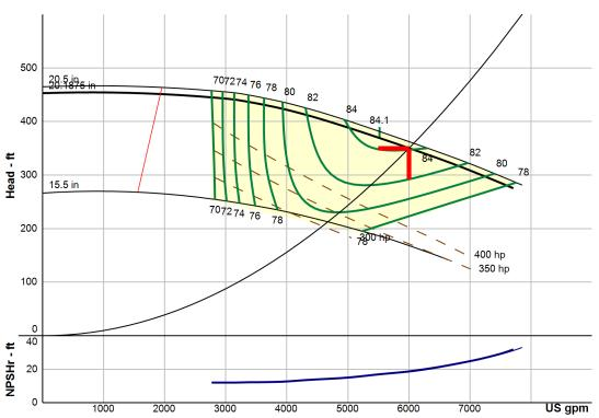
In accordance with the Hydraulic Institute Standards, pump is guaranteed for one set of conditions. Performance guarantees are based on shop test and when handling clear, cold, fresh water at sea level and at a temperature no greater than 85 degrees F. Suction lift must not exceed that shown on curve.
